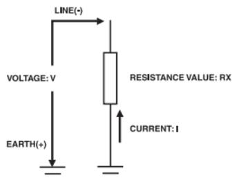
Terminal connection of insulation resistance test
