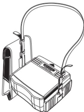
Pass the strap through the buckle, adjust the strap for length and secure.
