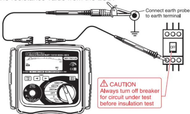
With the test probe still connected to the circuit under test, release the test button to discharge capacitance in the circuit after measurement.
